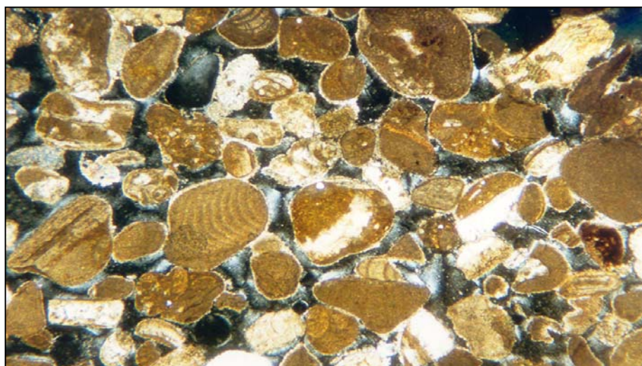
Figure 2.25 - Dune deposit is composed of a grainstone with well rounded fragments of molluscs, red corallinae algae, echinoids, bryozoan, benthic foraminifers, intraclasts; detrital grains are rare.
